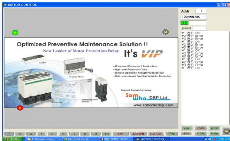
5) In this stage,if communication port to be run in "samdsp" is not matched with it in your PC, errored message in right column is shown, then user can preset right port number and bps in pop-up window that is shown by pressing "COM" button
