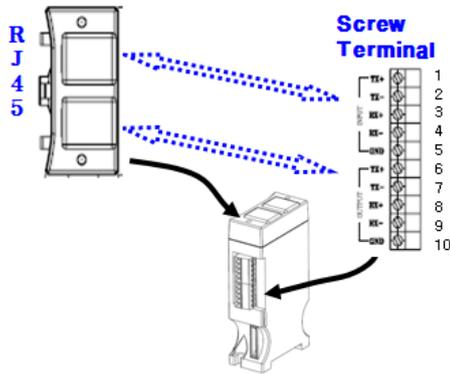
**Communication Module/Serial connection through RJ45 or Terminal**
