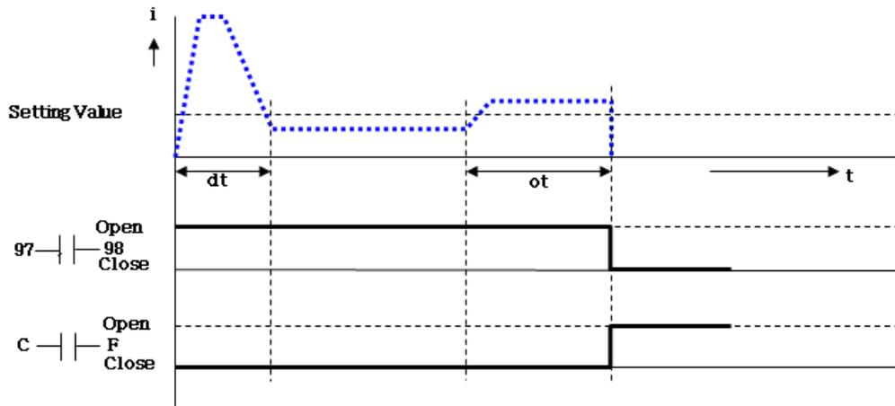
Shock/Stall Protection:AUX is selected for exclusive output for shock in "Au-o" mode
