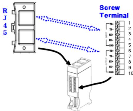
**Communication Module/Serial connection through RJ45 or Terminal**
