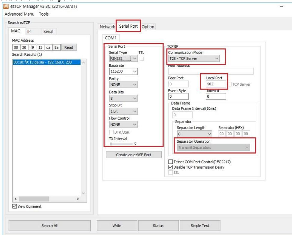
**4. make a store after input necessary information inside “option” menu, also “telnet” and “IPv address search” must be selected. Finally make a store as clicking “write”**
