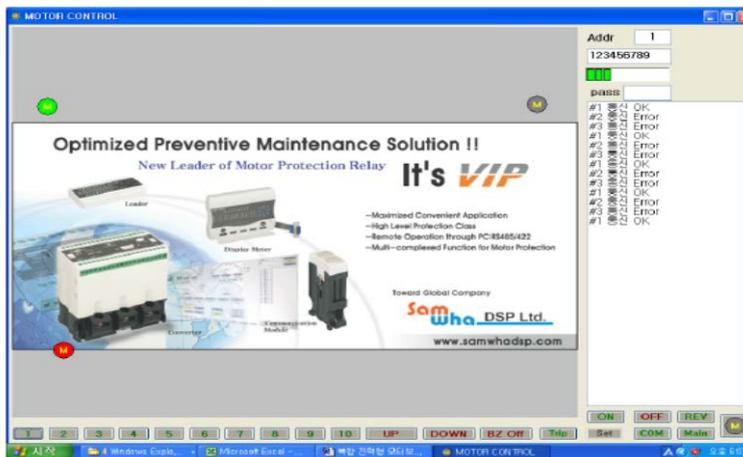
5) In this stage,if communication port to be run in “samdsp” is not matched with it in your PC, errorred message in right column is shown, then user can preset right port number and bps in pop-up window that is shown by pressing “COM” button
